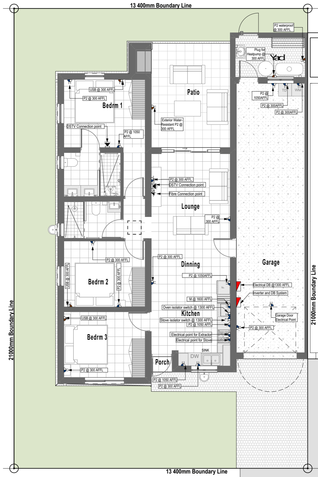
3.2 Electrical Plug Layout (G3) 1:100
