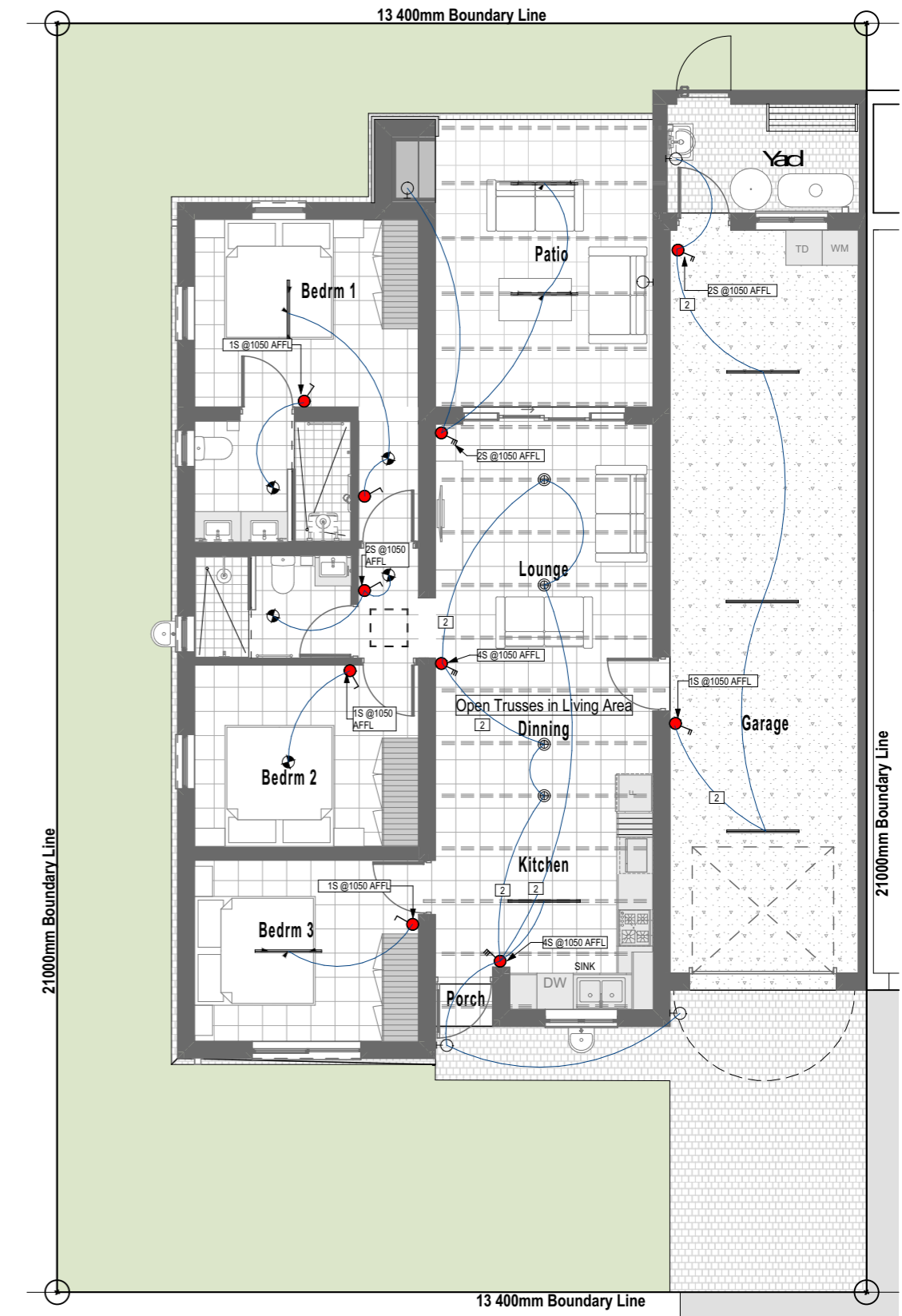
3.2 Light Fitting Layout (G3) 1:100
