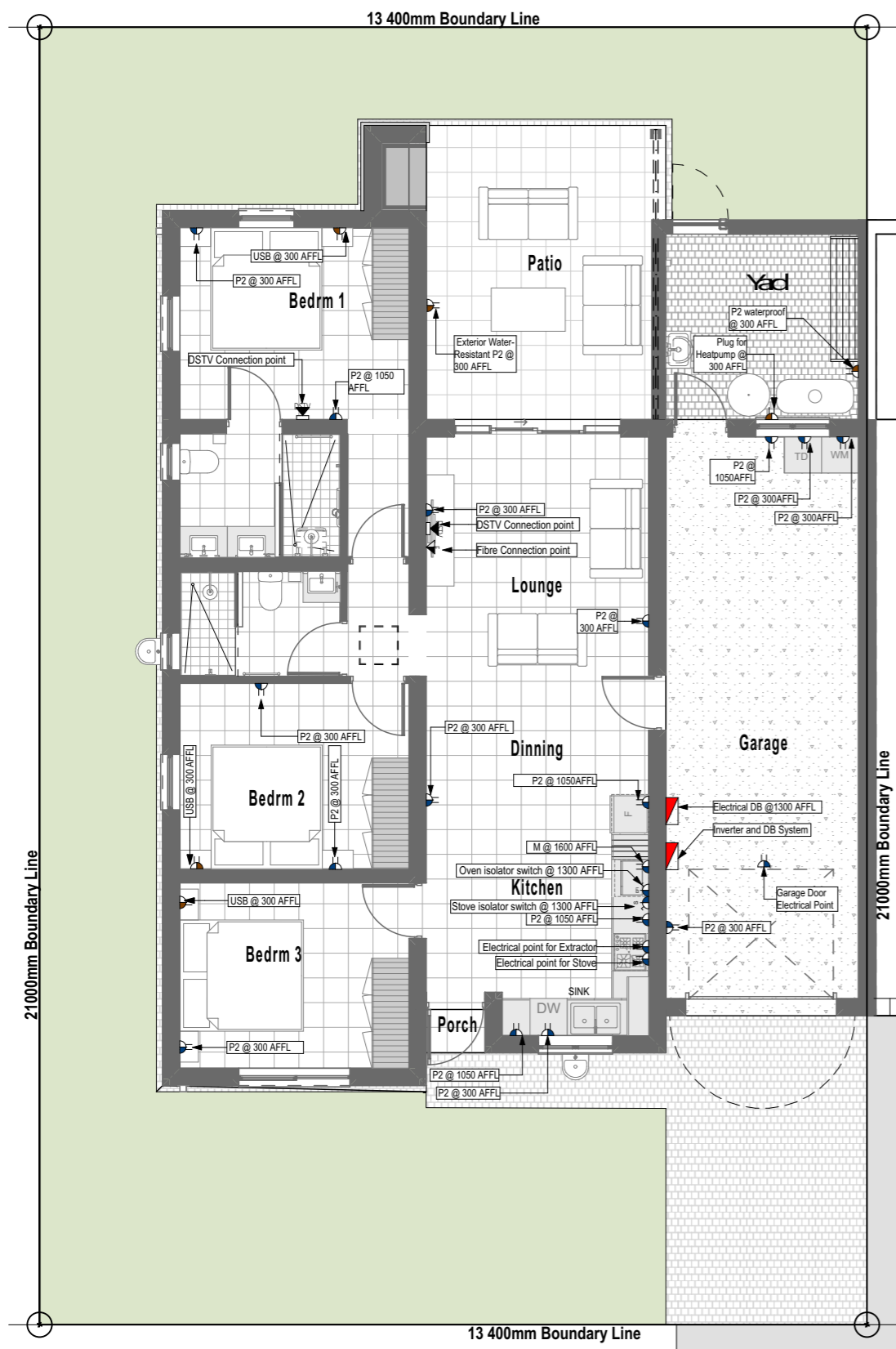
2.2 Electrical Plug Layout (G2) 1:100
