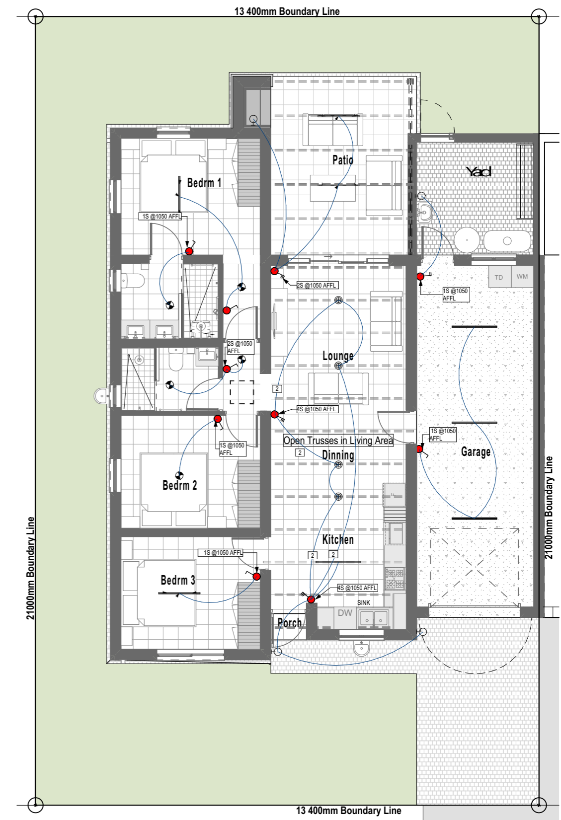
2 2.2 Light Fitting Layout (G2) 1:100
