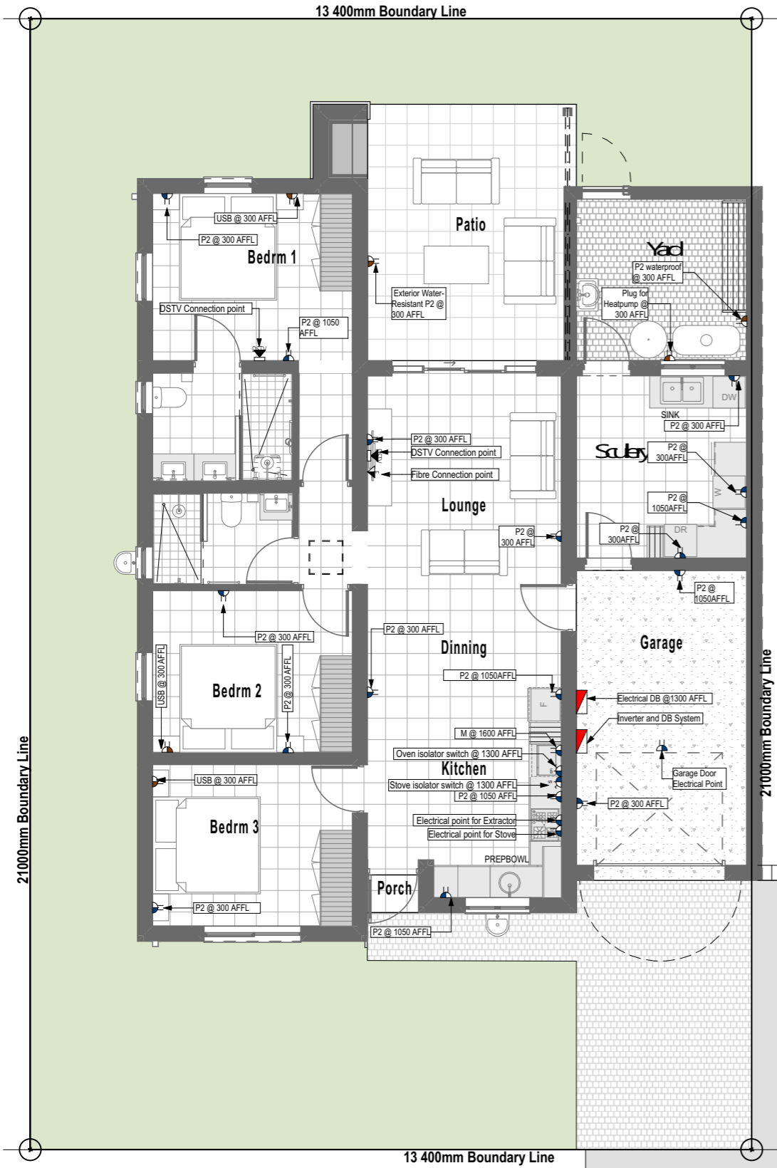
2.2.S Electrical Plug Layout (G2 - Scullery) 1:100
