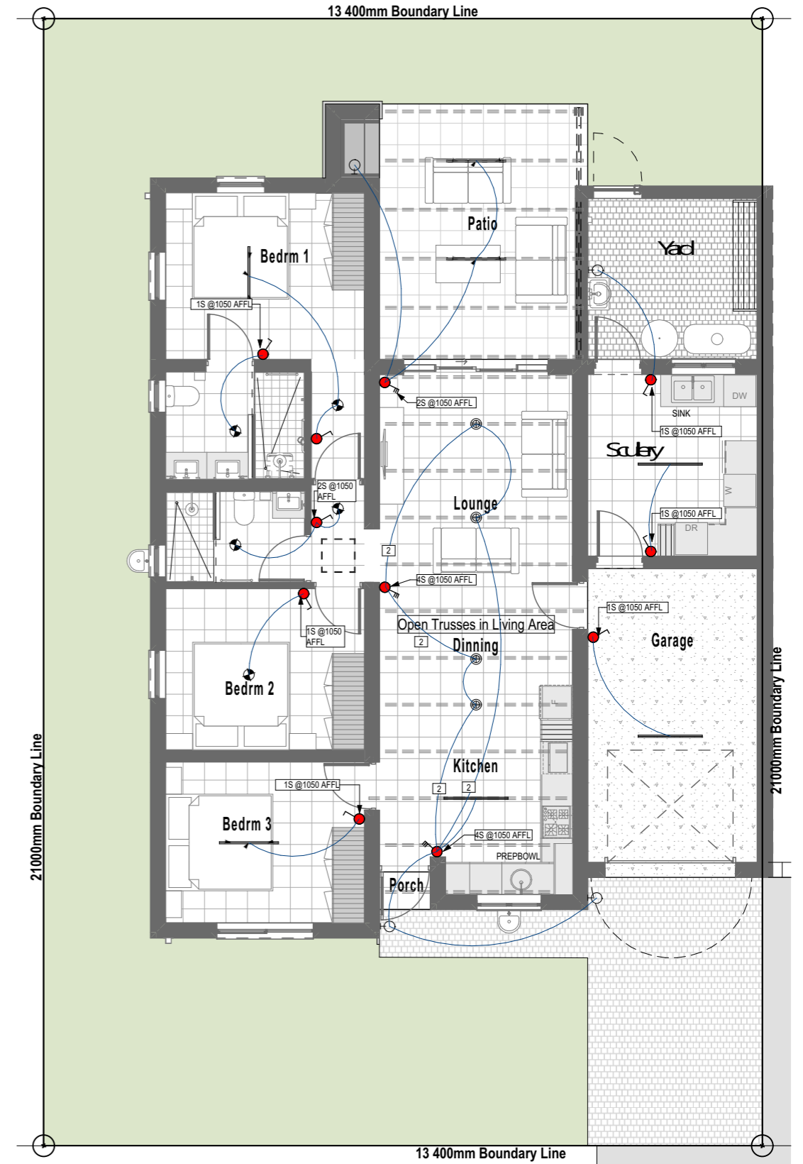
2 2.2.S Light Fitting Layout (G2 - Scullery) 1:100
