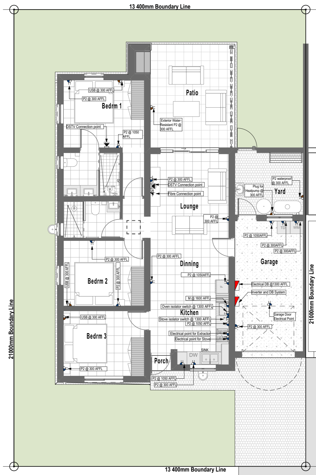
1.2 Electrical Plug Layout (G1) 1:100
