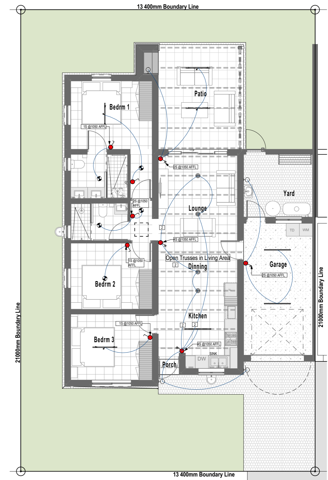
2 1.2 Light Fitting Layout (G1) 1:100
