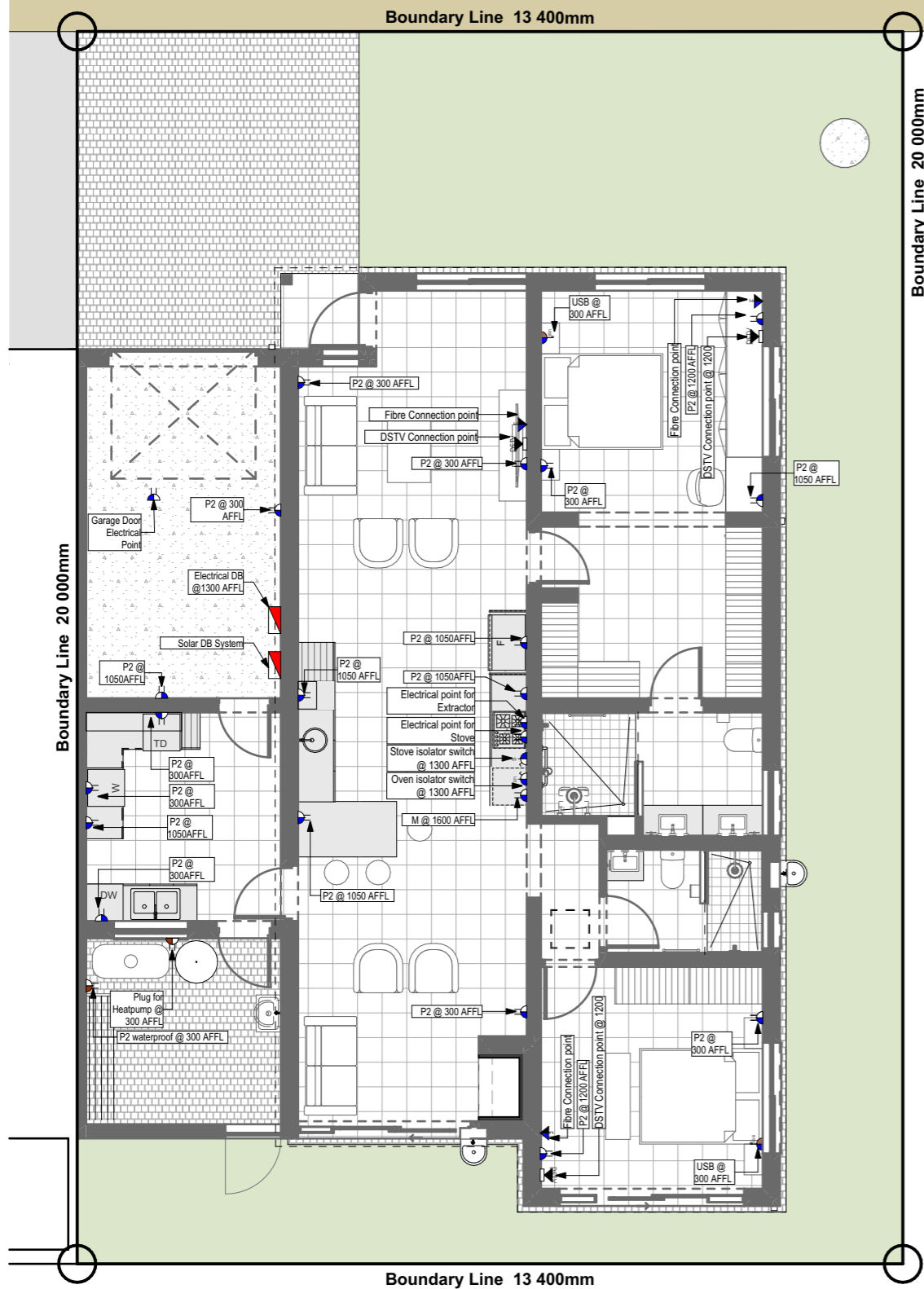
2.2.S Electrical Plug Layout - (D2-Scullery) 1:100
